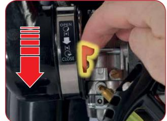
Move the choke lever downwards to the closed position. For cold starts, make sure the choke lever is closed.
