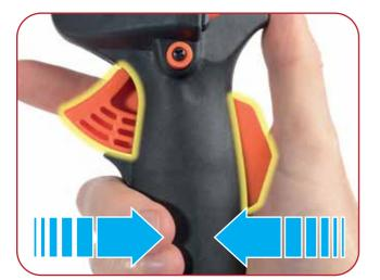
To use the throttle correctly you are required to unlock the throttle trigger by using the throttle lock enabling you to utilize the throttle trigger to increase the revs to the engine.
