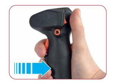
With the throttle trigger now unlocked use your index finger to activate the throttle and increase the revs to the engine.
