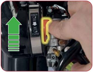
Move the choke lever upwards to the open position. For warm starts the choke lever should be open.
