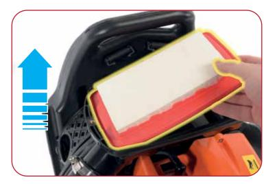
Remove the filter from the filter housing. The filter can be cleaned with lukewarm water and mild soap. Rinse well with clean water and allow to dry fully before replacing it.
