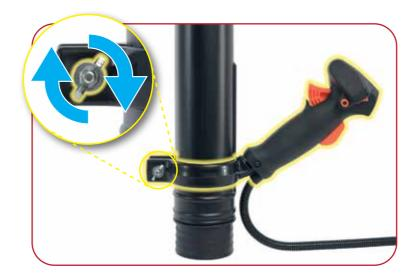
With the throttle assembly aligned with the centre rail, slide the throttle assembly all the way to base of the throttle tube. Tighten the wing nut to keep the throttle assembly in place.
