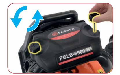
Remove the air filter retaining knobs. Turn them in an anti-clockwise direction then pull them out of the air filter cover.
