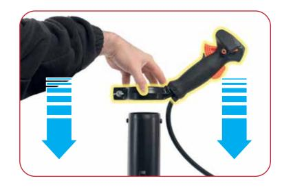
Loosen the wing nut on the throttle assembly and slide it on to the throttle tube. Rotate the throttle assembly so it fits over the two lugs on the end of the throttle tube.
