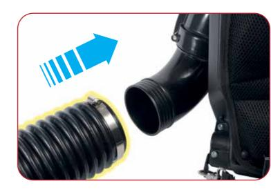
Attach the flexible tube to the elbow on the main body of the machine. It may take some force to get the flexible tube connected to the outlet.
