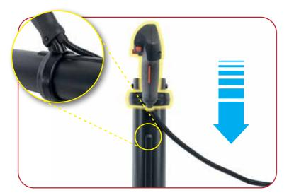
Rotate the throttle assembly again and align it with the centre rail on the throttle tube.
