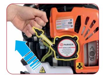
Place the machine on the ground and hold firmly in place. Then pull the starter recoil slowly until you feel the resistance.
