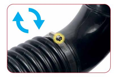
Secure the flexible tube to the elbow using the tube clamp provided. To tighten the clamp turn the screw in a clockwise direction.
