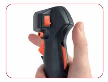
Half throttle is now set and the engine will remain revving at half throttle until the auto rev switch is disengaged or the machine is turned off.
