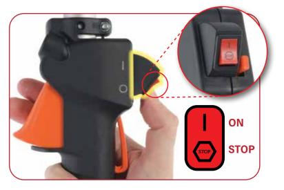
Turn the engine off by pressing the On/Off switch to position "O" or "STOP" as illustrated above. This will cut power to the engine. The switch will automatically return to the On "I" position.
