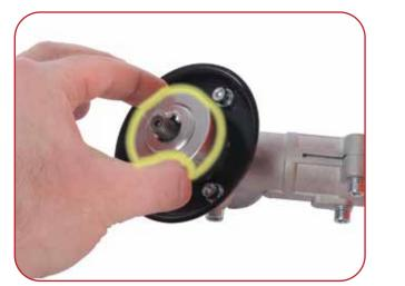
Install washer "A" as illustrated above. Align the washer with the hole on the spool collar. The purpose of this washer is to enable tightening of the nut by locking the hub. 2 LOCK HUB
