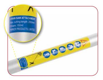
Locate the Chainsaw attachment pole which can be identified by the identification sticker.
