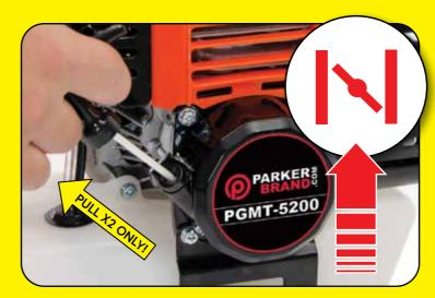
Make sure that the choke is **CLOSED** (UP ♠ CLOSED POSITION)
