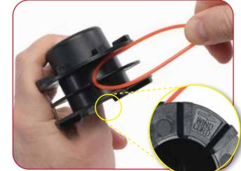
Open the spool by pressing one of the two clips to loosen the cover. Once loose firmly press the second clip and remove the spool cartridge from inside the housing.
