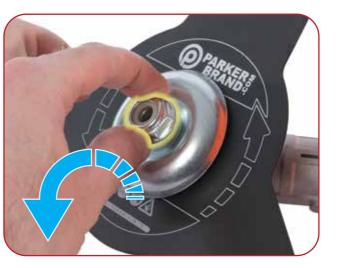
Install the hub nut as illustrated above to secure the blade to the shaft.
