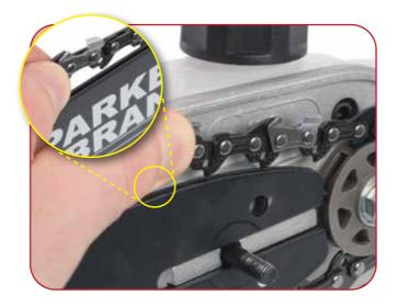
Loosely lay the saw chain into the groove on the bar start at the nose of the bar.
