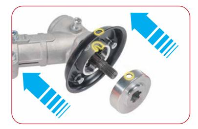
Align the holes on the collar, washer "A" and the axle. The areas highlighted above.
