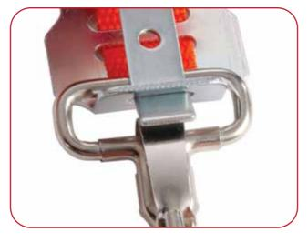
Place the release pin through the slot in the upper hook making sure that the pin passes over the lower hook.
