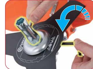
Place the allen key through the locating hole of the collar, through the hole of washer "A" and into the hub.
