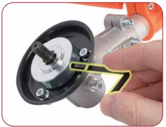
Lock the hub by inserting the allen key through the hole in the spool collar and into the hole in washer "A".
