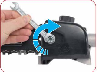
Once satisfied with the chain tension tighten the 10mm nut securely using the spanner provided within the tool kit.
