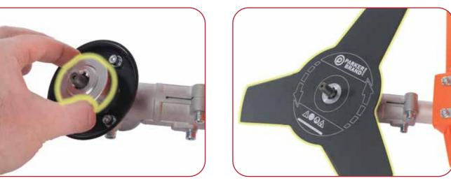
Install washer "A" as illustrated above. Align the hole in the washer with the hole in the spool collar. This is to help you lock the hub with an allen key later on in the process.
