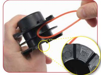
Secure the replacement spool line to the cartridge as shown The cartridge consists of two compartments in which the spool line needs to be wound. Wind in the direction shown on the body of the cartridge.
