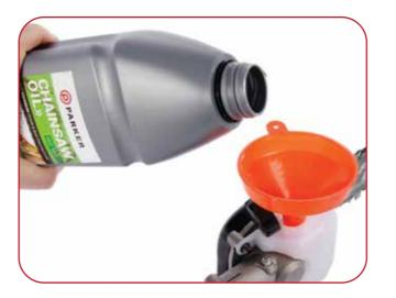
Fill the reservoir with chain oil. Use a suitable funnel to help poor the oil into the chain oil reservoir and prevent spillages.
