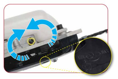
With the engine stopped, adjust the oil flow adjustment screw anti-clockwise to increase or clockwise to decrease.
