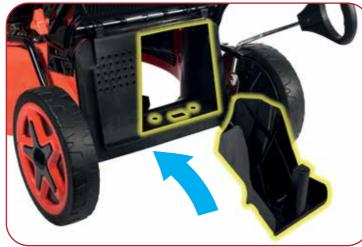
Remove the grass bag. Push the plastic mulching plug into the rear discharge chute until it is locked in place. Release the flap, it will close back to cover the mulching plug. 27 A
