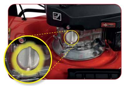
Locate the oil level dipstick, this will need to be removed to drain oil from the engine.
