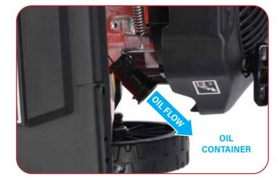
Allow the oil to drain from the engine and out of the oil filler neck into a suitable container. Always throughly clean the mower deck and any oil spillages before using the mower again.
