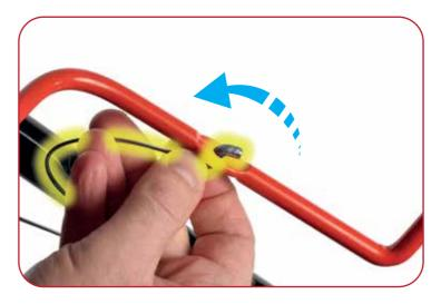
Disconnect the throttle cable by simply sliding the dog leg cable end in a curved motion through the hole on the lever.
