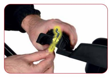
Thread the throttle cable through the cable guide hole located in the top of the drinks holder.
