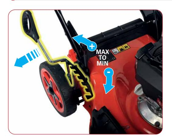
The cutting height is adjusted with the cutting height adjusting handle. Pull the handle out and select the desired cutting height. When released the handle snaps Into position.
