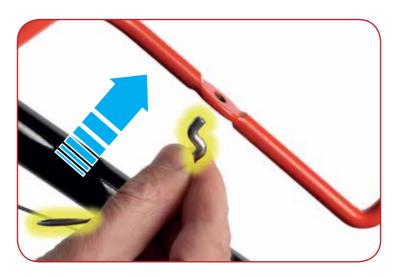
Re-thread the throttle cable through the hole on the throttle lever on the side where the cable has been threaded through the drinks holder.
