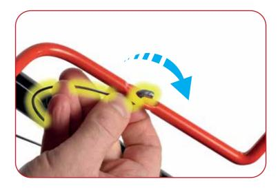
Secure the throttle cable by simply sliding the dog leg cable end in a curved motion through the hole on the lever.
