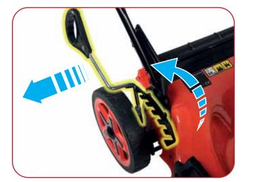
Before attempting to start the engine set the deck height to the highest setting. This will prevent the blade from catching on any uneven ground and make the machine much easier to start.
