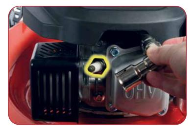
The sparkplug is easily accessible with the coil pack removed.
