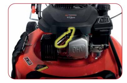
Locate and disconnect the coil pack from the sparkplug. This can be found at the front of the machine next to the exhaust.
