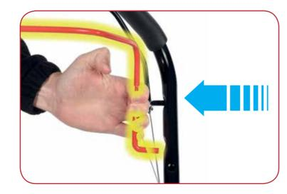
Pull the throttle lever away from the upper handle. The lever will pull free from the upper handle very easily, simply slide it freen from the opposite side.
