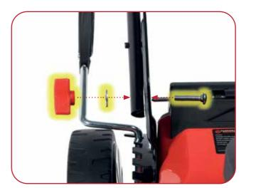
Thread the bolt through the square hole in the mower frame and through the lower round hole on the lower handle. Slide the washer on to the bolt and up against the lower handle followed by the red locking knob.
