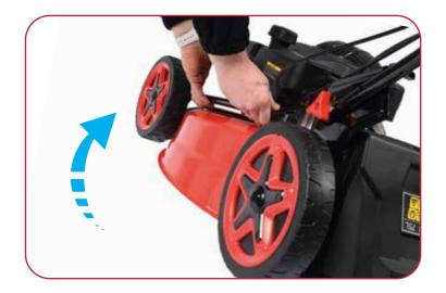
Have a suitable container ready to catch any oil drained from the machine. Carefully tip the machine fully on its side, making sure you follow the correct lifting proceedure to prevent injury.
