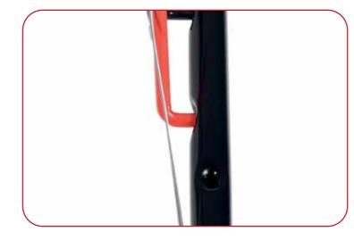
The throttle lever is now secured in place with the drinks holder and the throttle cable re-attached to the machine.
