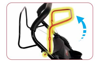
Stand behind the mower, pull the engine Start/Stop lever toward the upper handle. Place your other hand on the starter handle, pull the starter handle out approx.
