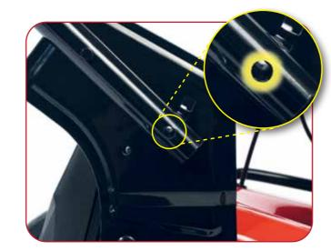
Align the lower round hole located on the lower handle with one of the square holes on themower frame.
