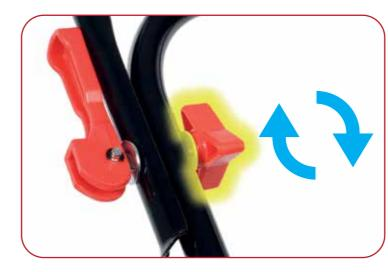
Tighten the locking knob by turning it in a clockwise direction. This process will need to be repeated on both sides of the handle.
