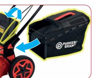
Lift the rear discharge cover with one hand and hook on the grass bag. Release the rear discharge cover to secure the grass bag in position.
