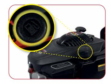
Remove the cap, check the fuel level. Refill the tank if the fuel level is low. Pour fuel carefully to avoid overfilling or spilling fuel.
