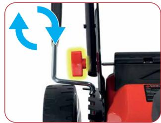
Tighten the red locking knob on to the bolt by turning it in a clockwise direction. Tighten until the lower handle is secured in place. This process will need to be repeated on both sides of the handle.
