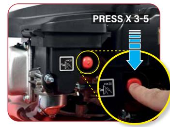
When starting a cold engine, press down the Primer fully 3-5 times.
