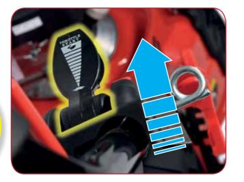
Put the throttle control lever in the START position before starting
