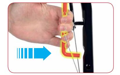
Guide the other pivot point of the throttle lever into the hole located on the upper handle on the cable side of the machine.
