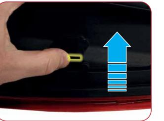
Unlock the side discharge cover by moving the locking machanism in an upward direction.
