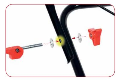
Assemble the locking knob as shown above. Thread the locking lever through both the upper and lower handle and secure in place by tightening the locking knob. This process will need to be repeated on both sides of the handle.
