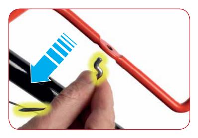
The throttle cable will now pull free from the throttle lever.
