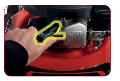
Remove the sparkplug using the sparkplug wrench provided. Dry the spark plug and then reinstall it. Follow the starting proceedure again carefully
