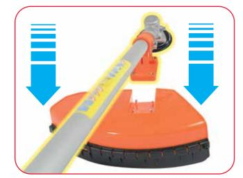
Align the lower guard to the lower guard attachment bracket located at the end of the lower shaft next to the hub.
