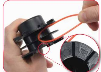
Secure the replacement spool line to the cartridge as shown. The cartridge consists of two compartments in which the spool line needs to be wound. Wind in the direction shown on the body of the cartridge.
