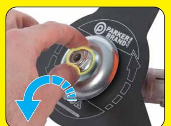
Install the hub nut as illustrated above to secure the blade to the shaft. The hub is reverse threaded so turn in an anti-clockwise direction to tighten.
