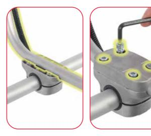
Loosen the four screws on the upper cap. Remove the upper cap and place the bull horn handle inside the recess.
