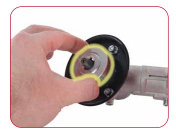
Install washer 'A' as illustrated above. Align the washer with the hole on the spool collar. The purpose of this washer is to enable tightening of the nut by locking the hub.
