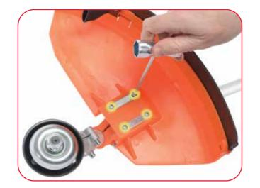
Attach the guard to the guard attachment bracket using the screws which are already installed in the lower guard, use the tools provided within the tool
