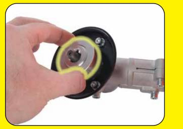
Install washer "A" as illustrated above. Align the hole in the washer with the hole in the spool collar. This is to help you lock the hub with an allen key later on in the process.
