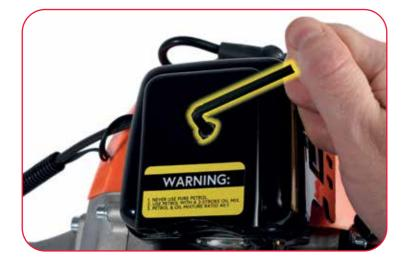
Locate the air filter cover on the machine. It is attached the carburettor with an allen head bolt. Use the allen key provided in the tool kit to loosen the bolt.
