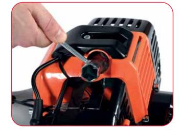
Remove the spark plug using the spark plug wrench. If the spark plug is fouled or is soaked with fuel, clean or replace.
