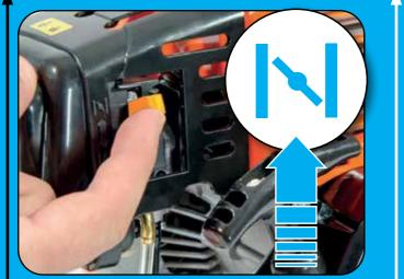
Perform a 'Cold Start' when the engine is cold. Move the choke lever into the upward position.
