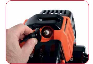
Disconnect the spark plug lead carefully by pinching the top and pulling away from the engine.
