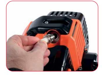
Install the spark plug and firmly tighten up with the spark plug wrench.
