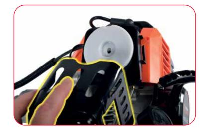
Remove the air filter cover. You will need to do this to gain access to the throttle cable and idle adjustment screw located on top of the carburettor.
