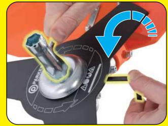
Place the allen key through the locating hole of the collar, through the hole of washer "A" and into the hub. Tighten the nut using the wrench provided, turning anti-clockwise until secured tightly.
