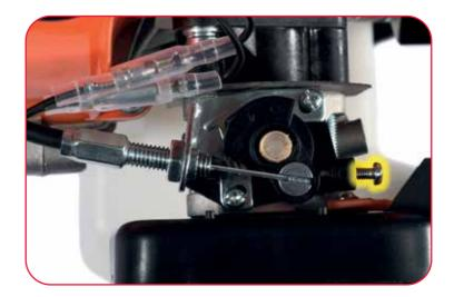
When the engine tends to stop frequently at idling mode, turn the idle speed adjuster screw clockwise. The idle speed adjuster screw is highlighted above.
