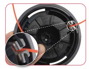
Place the cartridge into the spool cover and line up the ends of the spool line with the metal eyelets. Remove the spool line from the lugs on the spool cartridge and position them into the metal eyelets on the the spool cover.
