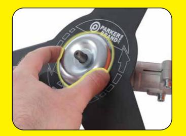
Install washer "C" as illustrated above. Washer "C" sits on top of washer "B".
