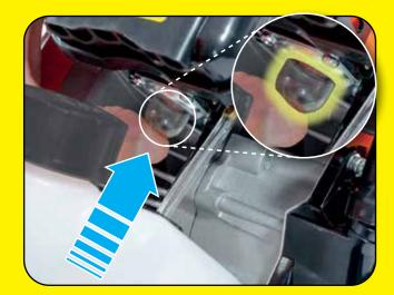
The engine switch is spring loaded. The default position of the switch is the 'ON' position.
