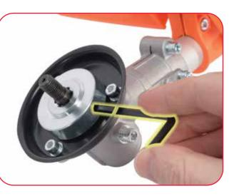
Lock the hub by inserting the allen key through the hole in the spool collar and into the hole in washer
