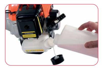
Always turn off the engine and allow it to cool down first . Fill the tank with the clean, fresh pre-mixed petrol and 2-stroke oil. Use a funnel if required to prevent any unnecessary spillages. Wipe up all spilled fuel completely. When refilling the tank, take a careful look around to make sure that there are no sparks or open flames anywhere nearby before refuelling. After refilling the tank replace the fuel cap.
