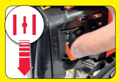
At this stage the choke must be OPEN.
