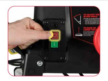
The red OFF switch (O) stops the machine.
