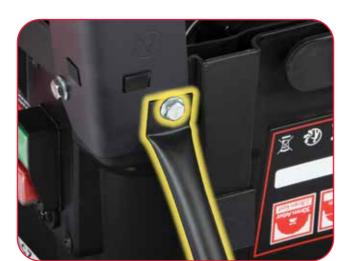
Attach the support struts onto the table side. You will have to remove the hex head screw holding the leg in place. Position and hand tighten.
