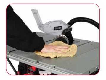
Only use a damp cloth to wipe down the table surface and any plastic parts.
