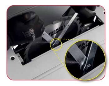
Use the hexagonal spanner to remove the outer flange and blade. Clear all the parts and the area where the blade sits of debris.
