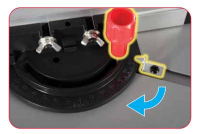
To set the angle that you desire simply loosen the red handle. Use the protractor scale and pointer to set the gauge to the angle that you require. Once the angle is set, tighten the red handle
