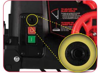
The overload protection is a feature that protects your machine in the event of the rated load for the machine is exceeded. If exceeded for some reason the machine will automatically cut out. To start the machine again press the over load protector as shown and the 'ON' button.
