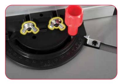
The adjustable face plate is held in the protractor base with two wing nuts - loosen to adjust and then tighten to secure.
