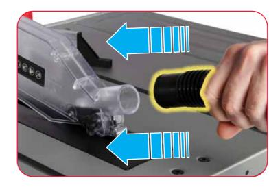
The extraction hose is a simple push fit. Fit the hose to the top of the guard as shown.
