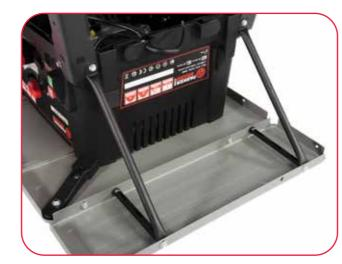
Repeat Process. Note that the Hole is oval to position as you like. Make sure the side panels are flush with the main table surface of the saw. You can use a straight edge to verify this.
