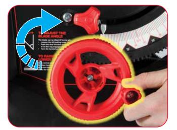
To raise the blade simply turn the wheel clockwise in the normal position.
