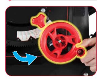
Push the turning wheel into the inner position so that it engages with toothed rack.
