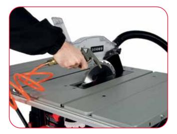
Use a workshop Air line or a vacuum to remove any saw dust from hard to reach places.
