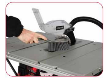
Use a soft brush to clear away any debris left behind from using the machine.
