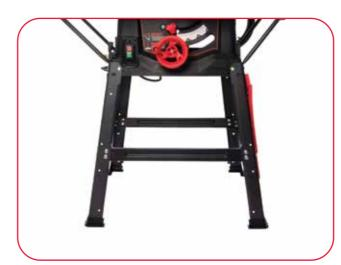
Turn table over to upright position. Leave to settle for a few minutes. Adjust as necessary to ensure the table is level and stands firm. Firmly tighten all screws using either a spanner or socket set. Do not over tighten.
