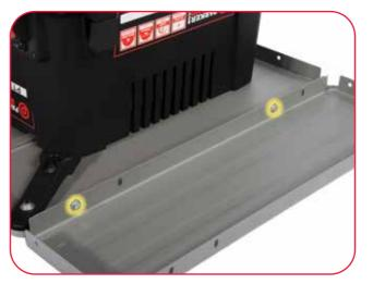
Identify the highlighted pre-drilled holes. Use hex head screws and flange nuts to fit the table extension. Pay particular attention to the holes used to attach the extension as if positioned incorrectly the next step will not be possible.
