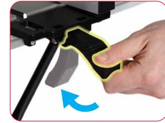
The locking lever, as previously mentioned, lifts and drops down to lock the rip fence into place anywhere along the length of the machine either side of the blade.
