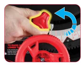
To tilt the angle of the blade (up to 45 degrees) turn the red locking knob as indicated to loosen.
