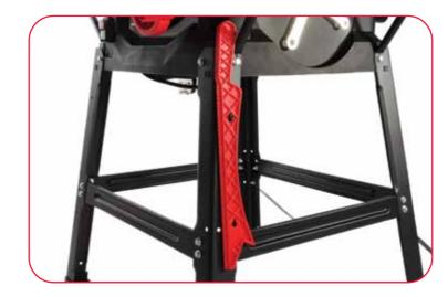
The push stick is stored on the right-hand front leg. Simply hang it on the hex socket screw cap held in place by the small nuts - check the what's in the box section.
