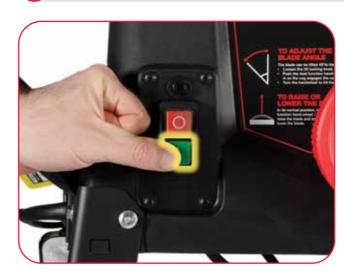
The green ON switch (I) starts the machine. Make sure the blade guard is positioned correctly before starting.
