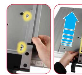
The rip-fence face plate can be repositioned if required. Loosen wing nuts and slide forward or backward as desired.
