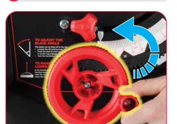
To lower the blade simply turn the wheel in its normal position anti-clockwise.
