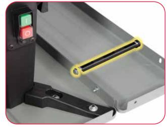
Using a hex head screw fix the support bars in place, tightening at the machine side by hand.
