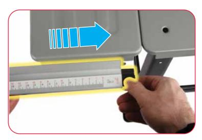
Slide the fence rail over the protruding bolts and position the rail centrally.
