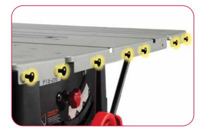
Attach all 7 coach bolts utilising the supplied flange nuts. (3 to the main body, 2 to each extension). Tighten by hand.
