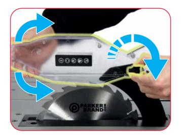
To adjust loosen the wing nut and move the blade guard into the position. The guard should be set at an appropriate level for the thickness of the material you are cutting.
