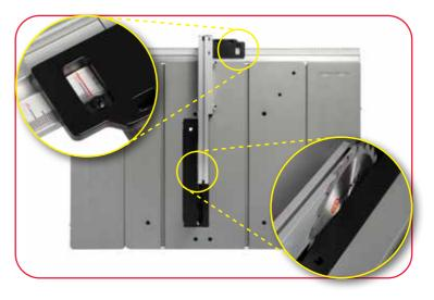
To adjust the fence rail correctly, place the rip fence on the fence rail. Position the rip fence so it sits flush against the blade. The dual read scale should read zero. If not reposition the rail until the dual read scale reads zero.
