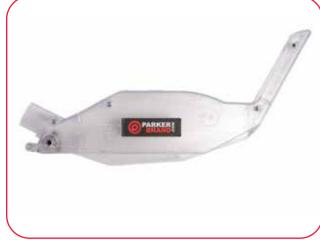
The top blade guard must always be fitted to the riving knife. The line at the top of the guard reflects the cutting line of the saw blade.
