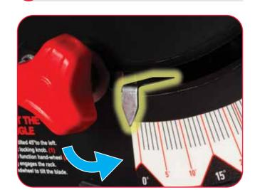
Adjust to the angle required. Making use of the protractor scale and pointer. Whilst accurate it is always recommended that any measurement is double checked before making a cut.
